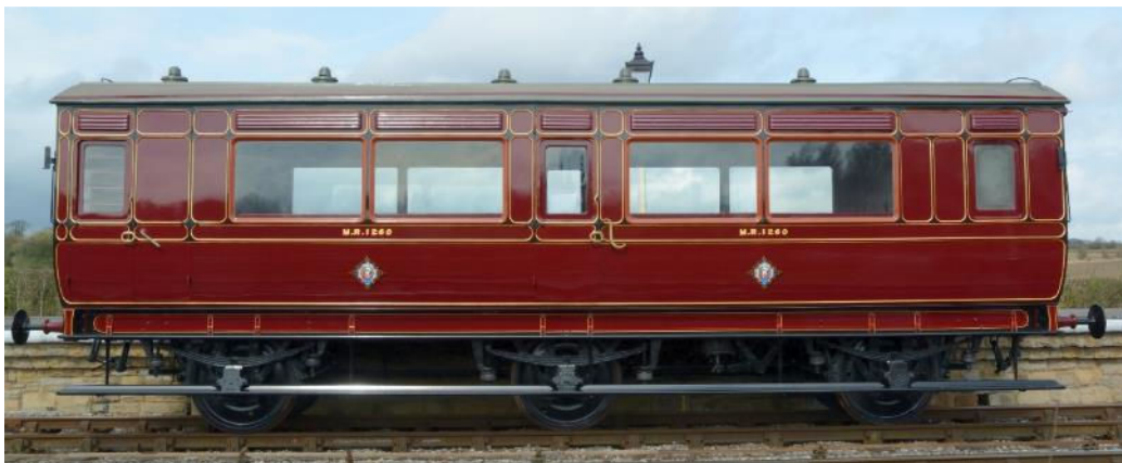
Midland Railway Party or Picnic Saloon Built 1890 in Derby. Six wheeled, one large compartment with four upholstered bench seats, a lavatory compartment, with a flushing WC and sink, and a luggage compartment. Used for group travel.
