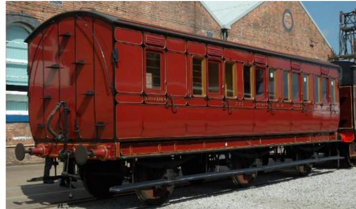
Midland Railway Brake Carriage Built 1888 in Derby. Six wheeled, three passenger compartments, upholstered seats, and a Guard's compartment with space for luggage and light goods.
