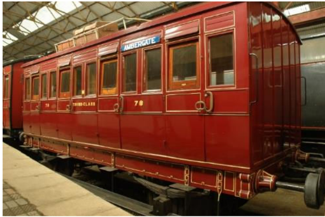
The oldest surviving Midland Railway Carriage Built about 1868 in Derby. Four wheeled, four passenger compartments, wooden seats and luggage accommodated on the roof.
